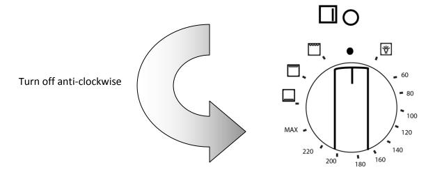
When selecting a temperature between 60°C and MAX the half oven will automatically be set to conventional oven mode. When selecting "bottom bake", "top bake" and "grill" functions the temperature will be automatically set to high. To turn the oven off the control knob must be turned anti- clockwise to the off position. Do not force the control knob the other way as it will damage the appliance.
