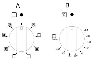
When using the main oven, you can select your desired (B) temperature according to the cooking function selected (A)
